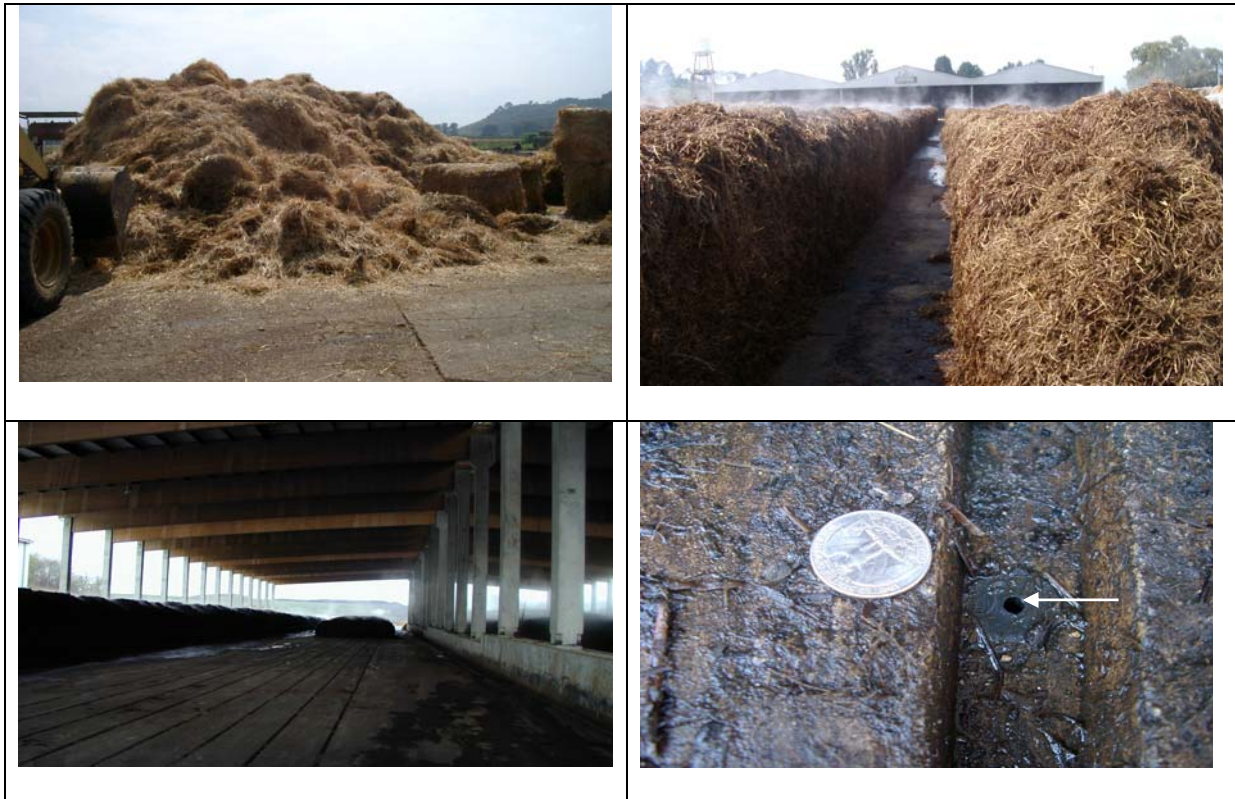
Figure 1. Loose straw ready for incorporation into compost windrow (top left); compost windrow (top right); aerated Phase I compost wharf under roof (note grooves in concrete, bottom left); groove showing aeration nozzle (bottom right, arrow).
